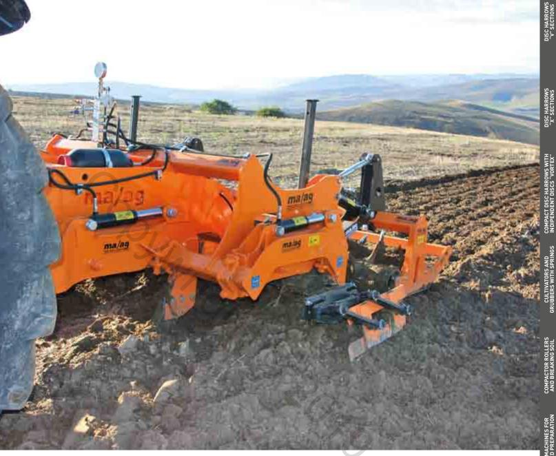
Version with double spike roller, tube diam.220 mm, manual regulation
