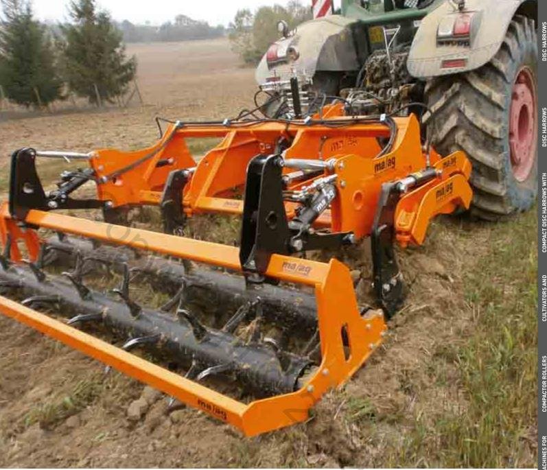
Version with double spike roller, tube diam.220 mm, hydraulic regulation
