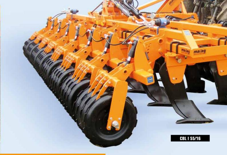
EQUIPMENT WITH PRESSED STEEL ROLLER, WITHOUT DOUBLE BREAKING DISCS
