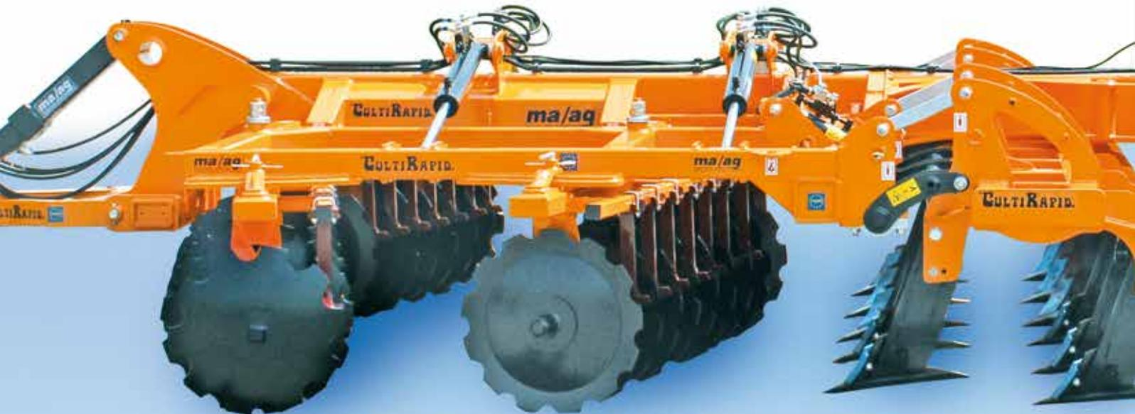
Double toothed rounded discs, realized with boron steel discs, mounted on a steel shaft and swiveling supports with double conical bearings, system ma/ag. The disc sections are arranged on “rhombus” shape, patented system ma/ag. Mechanical adjustable regulation in different positions.
