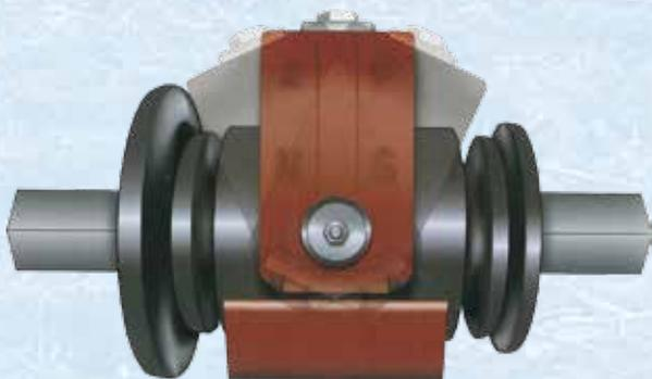
On the Cultirapid PRO we are using swiveling supports with two conical roller bearings (for absorbing in addition to the vertical charge also the horizontal actions), provided with an interchangeable protection carter.
