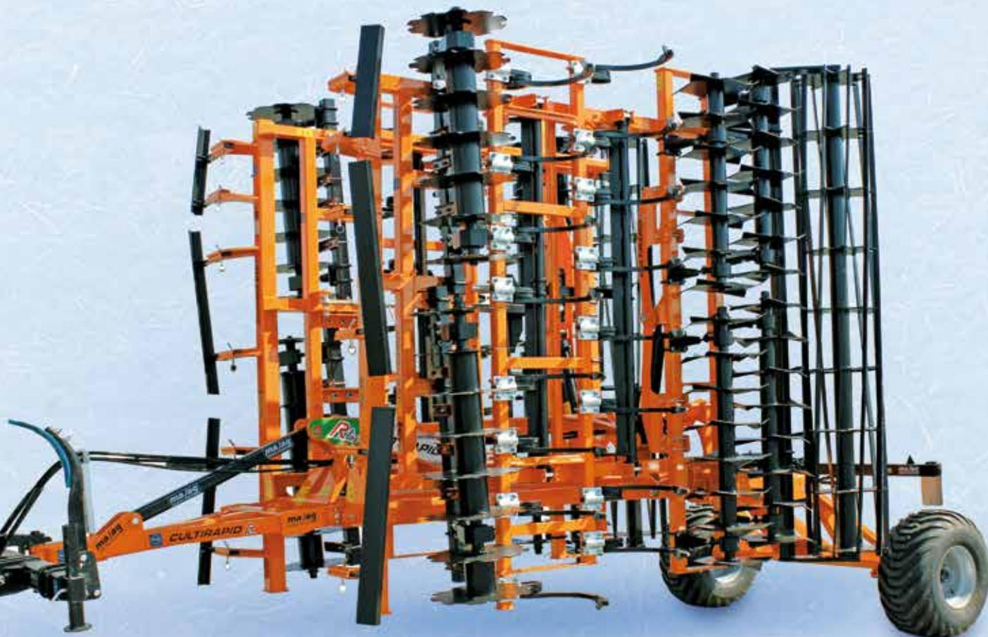
**CHÂSSIS PLIANT POUR CIRCULATION SUR ROUTE DIMENSIONS HORS-TOUT POUR TRANSPORT 2,55 M**
