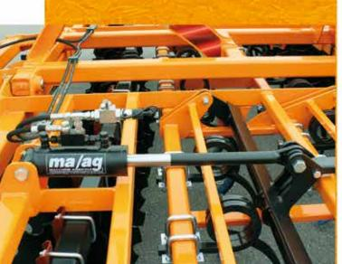
Mechanical change by adjustable III point linkage.
