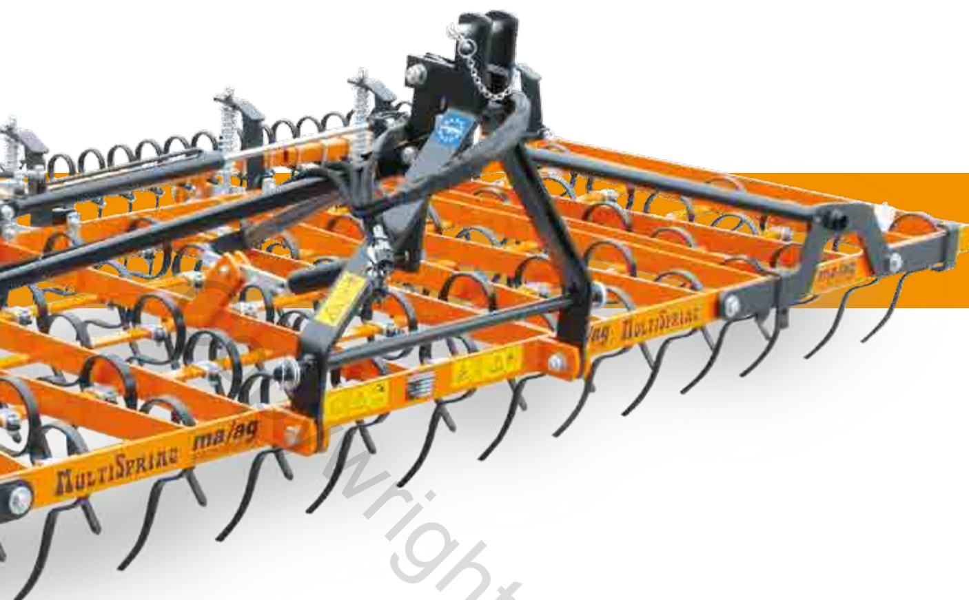
For the RD versions with double rear roller it is recommended the mounting of the hydraulic system for folding lateral parts
